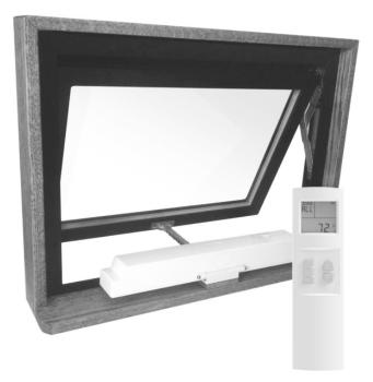
Solar Smart is a battery powered, solar charged, remote operated, chain drive opener system – designed for use in awnings, hopper windows, and skylights. Solar Smart is designed to be used without any additional power and wiring from the building. The operator is powered by a Lithium battery pack that is recharged from the external solar panel; an optional AC adapter is included. Solar Smart was engineered to feature ultra-low power consumption while in idle state, and in use.
