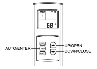
• Using the operator requires that it has been paired to the remote. Refer to Initial Remote Setup and Configuration.
