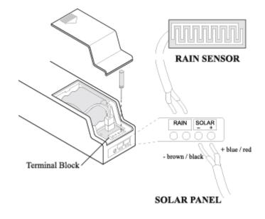
**NOTE:** If the wires for either the Solar Panel or Rain Sensor were installed then removed, the internal locking tabs may need to be re-opened to allow the wires to be fully re-inserted. To do this, simply use a strong pin, heavy paper-clip, a finishing nail or any similar small object – and insert the pin into the wire hole and press firmly but gently until you either feel the click of the locking tab opening, or you are certain that the wires can be inserted fully. Repeat for each wire hole.
